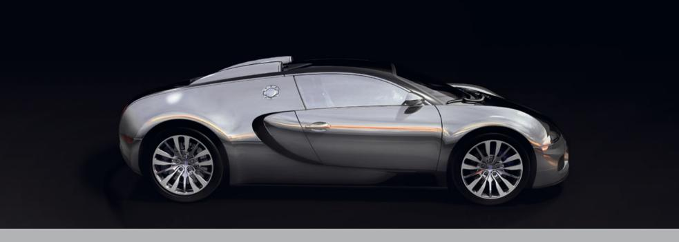
The EB 16.4 Veyron Pur Sang is a two-tone study of pure material showing the car's true essentials: carbon and aluminium. The clear-coated carbon monocoque holds the engine and the passenger cell, while the polished aluminium panelling is enhanced by reflections in the sculpted bodywork.
